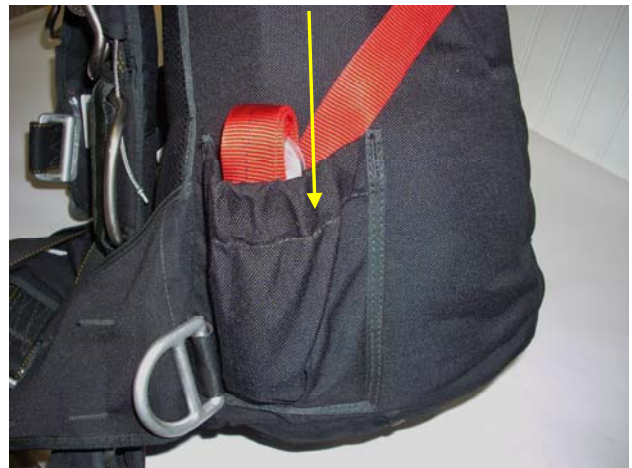
Stow the remainder of the Static Line into the pocket on the side of the Container.
