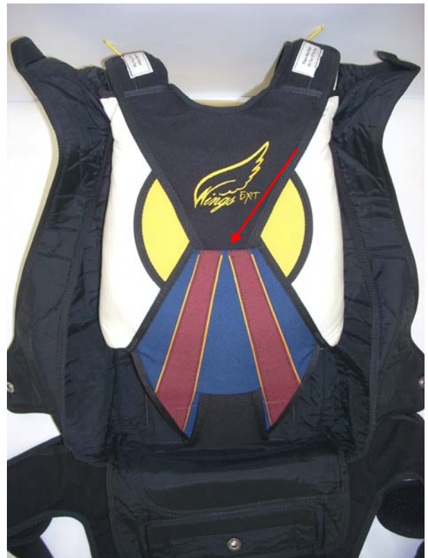
Tuck the Top Reserve Cover Flap into the Bottom Reserve Flap pocket.
